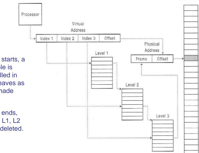
When a process starts, a new L1 page table is allocated, then filled in with L2 and L3 leaves as new pages are made valid.
